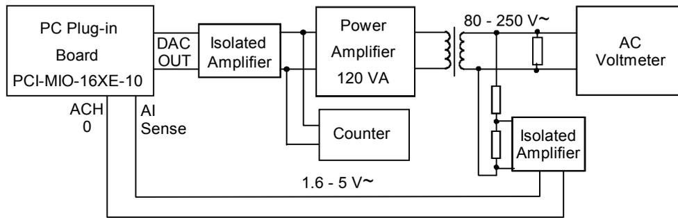
Fig. 5. Block diagram for calibration process
