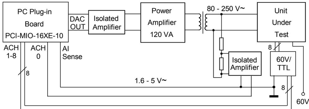
Fig. 1. Block diagram of the developed system
